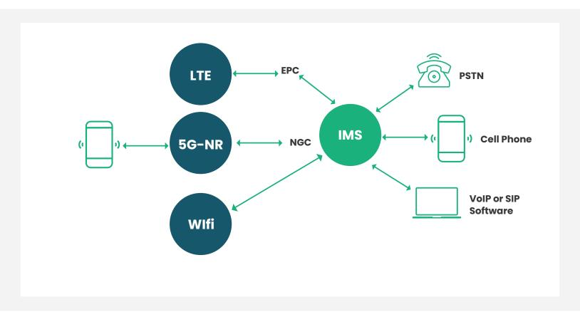
5G networks will use Voice over New Radio (VoNR) – as part of their new architecture to offer significantly better sound quality and lower latency. VoLTE, VoWiFI and Vo5G are just technologies which describe the technical aspect of the connection between UE (user equipment) and IMS core. All IMS threats will also be present in any of these technologies. Below are common IMS threats.
